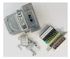
The pin version SUB-D15M-Weber was specially designed for the ultrasonic generator LC series from Weber.
